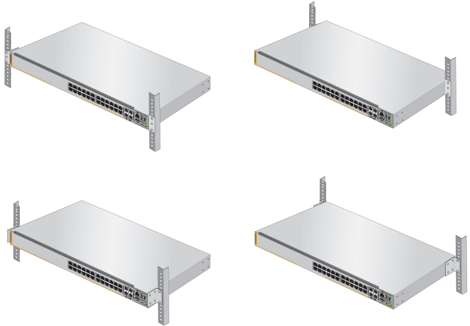
Figure 28. Switch Orientations in an Equipment Rack
