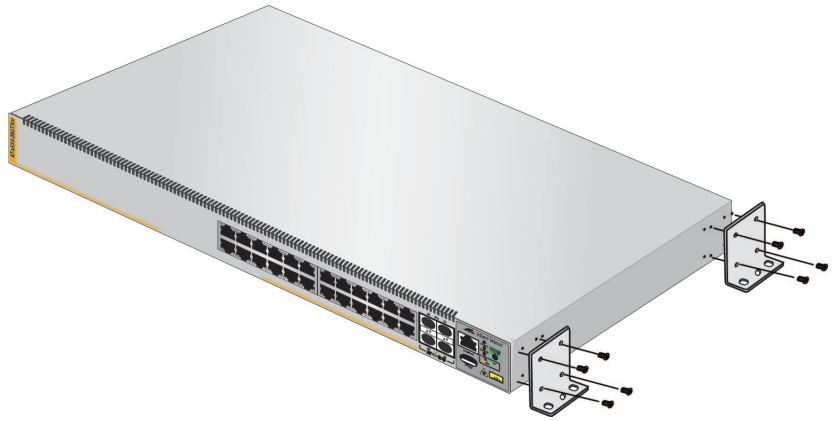
Figure 35. Installing Two Brackets on the x530-28GTXm or x530-28GSX Switch
